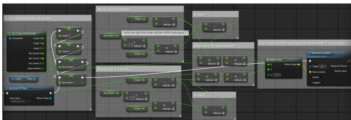
Figure 9: A snippet from the hammers movement logic where its location is set using the coordinates of a hidden plane. This displays the confusion around using maths in blueprints
